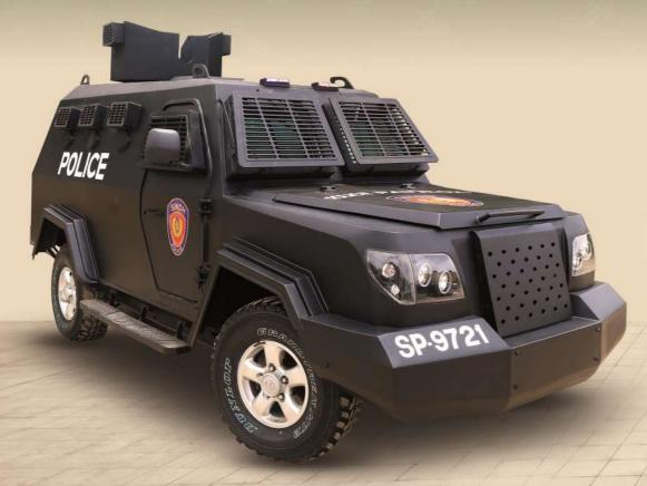
Sagr Pak Armoring Pvt Ltd is proud to introduce the Armored Personnel Carrier (APC), a vehicle armoring solution specifically designed and engineered for Law Enforcement personal transportation in Pakistan. This is built on a heavy duty chassis, equipped with a powerful 200 horsepower, 4.5L\V8 engine, and 5 –speed Manual transmission @3400rpm.
